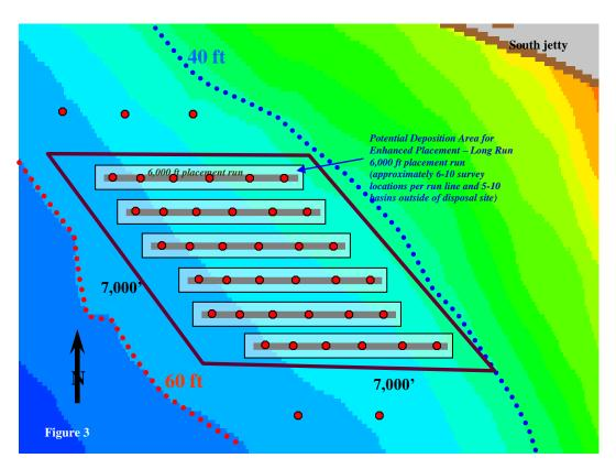
Figure 1: Approximate location of minimum number of survey points (figure modified from USACE).
